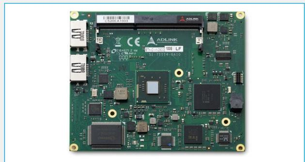
**Figure 3: Typical ETX® module**
