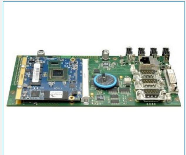
**Figure 1: Typical implementation using a COM**
