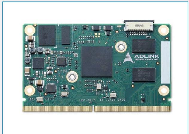
**Figure 5: Typical SMARC module**
