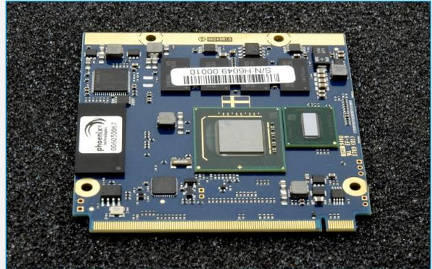
**Figure 4: Typical Q7 module**
